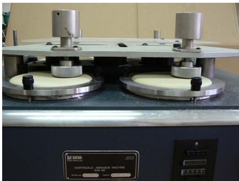
Martindale abrasion machine fitted with leather test pieces and control/soiling cloth materials in the head unit.
