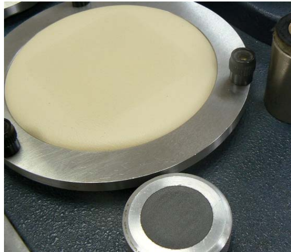
3,500 soiling cycles on conditioned/protected leather
