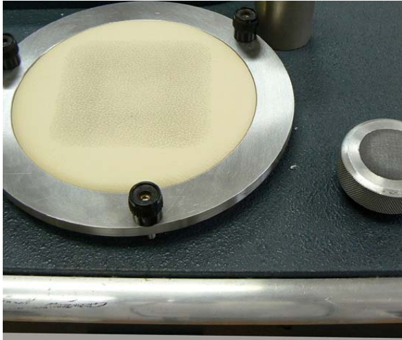
3,500 soiling cycles on untreated leather
